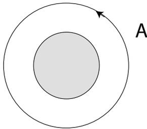
Figure 2: Cross section view of the solenoid, with a path around it in a region with vector potential  $\mathbf{A}$ .
